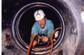
Pressure Test Seal
