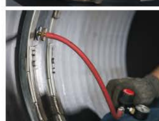
Pressure Test Seal
