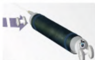
3. Install Packer's Rear Wheel Assembly
