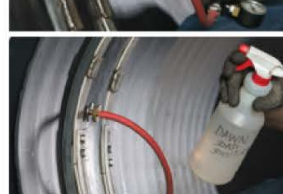
Pressure Test Seal
